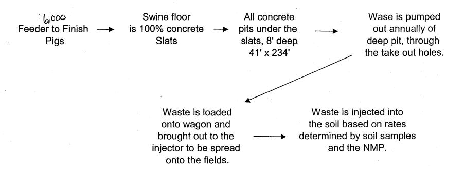
This site houses 10,000 wear to finishes hogs. The 234 Building has 8' deep pits and there are 5 of these Buildings. The 214' buildings also have 8' deep pits and there are 4 of these buildings. The concrete is reinforced with rebar. There are 4 pit pumps on one end & I on each side. PTO driven centrificals pump the name from the pits. These buildings are 100% total stats. Pit Sizes <- 234'-> 1200 Hd. Bouns Eapacity 1000 Hd. total capacity. bains 214-7
